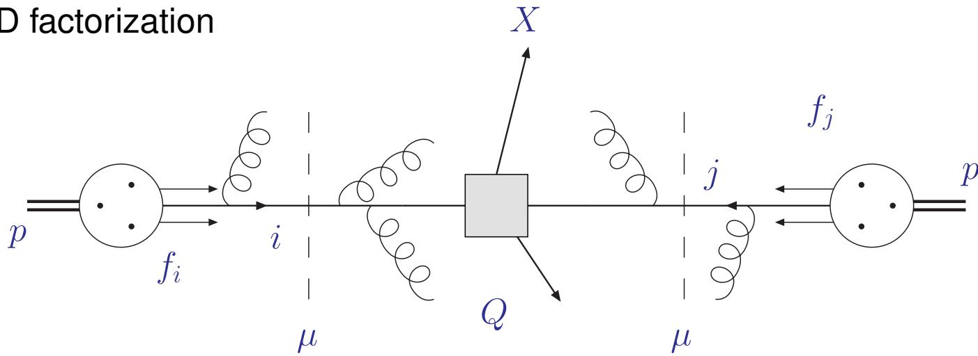
$$\sigma_{pp \rightarrow X} = \sum_{ij} f_i(\mu^2) \otimes f_j(\mu^2) \otimes \hat{\sigma}_{ij \rightarrow X} (\alpha_s(\mu^2), Q^2, \mu^2, m_X^2)$$
