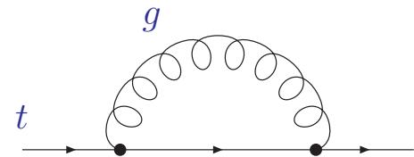
$$\Sigma^{(1),\text{bare}}(p, m_q) = \frac{\alpha_s}{4\pi} \left( \frac{\mu^2}{m_q^2} \right)^\epsilon \left\{ (\not{p} - m_q) \left( -C_F \frac{1}{\epsilon} + \text{fin.} \right) + m_q \left( 3C_F \frac{1}{\epsilon} + \text{fin.} \right) \right\}$$
